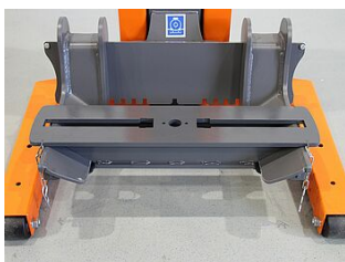
EHB907TRT412TR01-38 5 Basic cross beam 880 mm, tractor support at front
