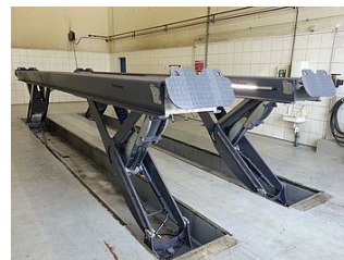
HDSF07DUROPLEX-XX Special coating in addition to galvanizing
